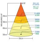
LED Light, 24V/6W, 25°Lens SL9 LED Light, 24V/6W, 40° Lens
